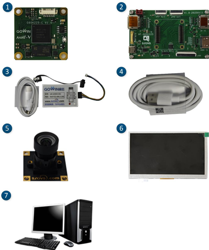
Figure 4-7 Hardware Composition of SC2210 Color Exposure 1-lane LVDS Screen Display Project
