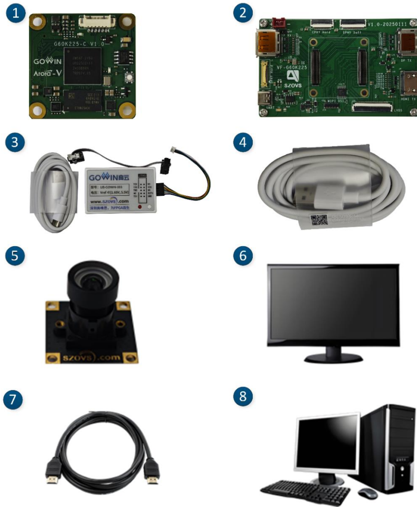
Figure 4-5 Hardware Composition of SC2210 Color Exposure 1-lane HDMI Screen Display Project
