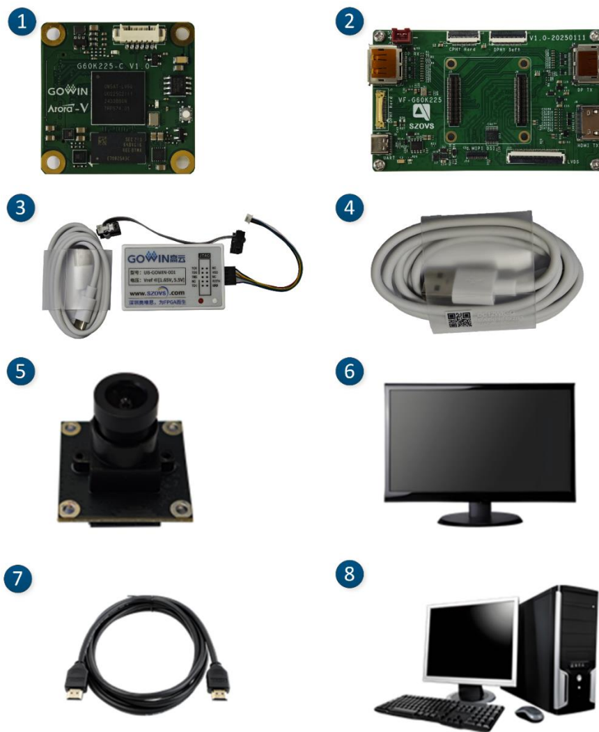
Figure 4-1 Hardware Composition of SC130GS Black-and-White Exposure 1-lane HDMI Screen Display Project
