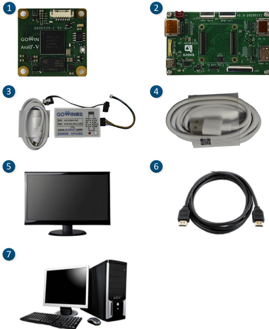
Figure 3-17 Hardware Composition of 1920*1080@60 DDR3 Image Cache and HDMI Screen Display Test
