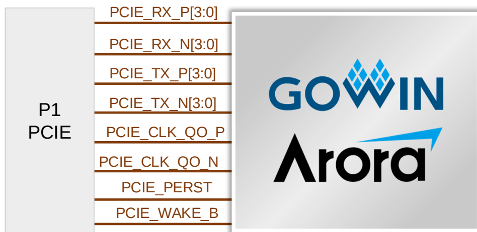
Figure 3-8 Connection Diagram of PCIe Interface
