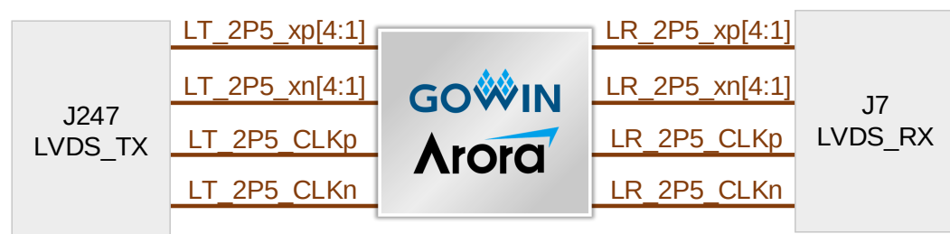
Figure 3-10 Connection Diagram of LVDS Interface
