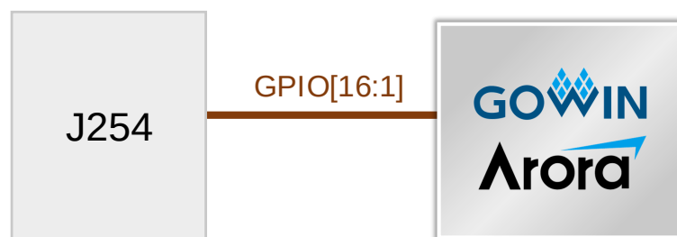
Figure 3-11 Connection Diagram of GPIO Interface
