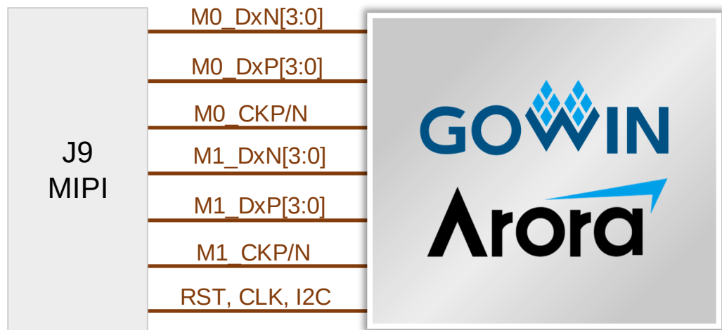
Figure 3-7 Connection Diagram of MIPI Interface
