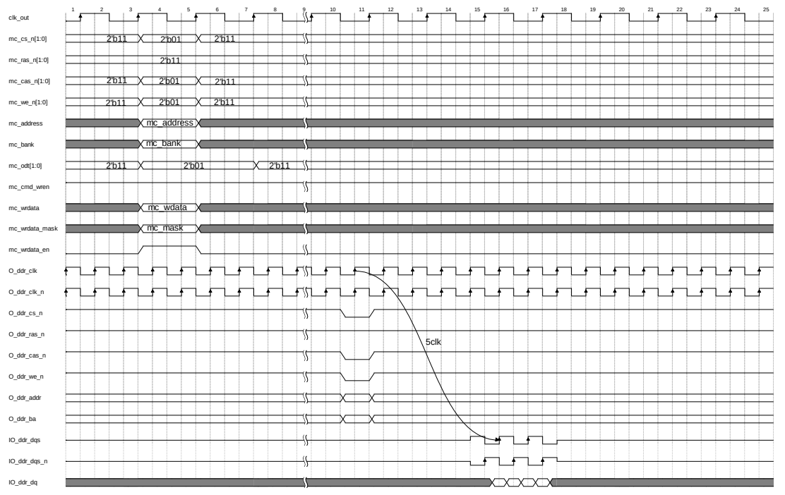
Figure 3-16 Timing Diagram for Write Data with Burst Length=4, CL=6,AL=0
