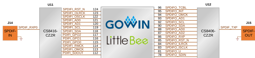
Figure 3-5 SPDIF Interface Connection Diagram
